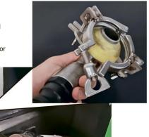
◀FFED has taken care to develop 2 connectors which allow almost all DPF assemblies on the market to be connected to the machine.
