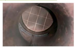
▲ Once treated by the Carbon FAP, the filter is restored to its original appearance and full performance. It's important to note that the silicon carbide composing the DPF is a material highly resistant to thermal and mechanical shocks, allowing it to be reconditioned - theoretically - as many times as the vehicle's lifespan requires.
